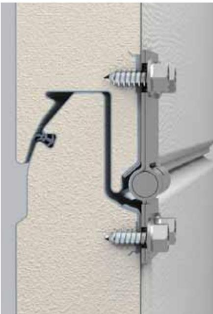
Self-tapping screws are positioned at the junction of the of external and internal sheets (**4 layers of metal**) which makes the fixing more durable. Reliable connection of steel sheets prevents panels from delamination in case of the door closing abruptly.
