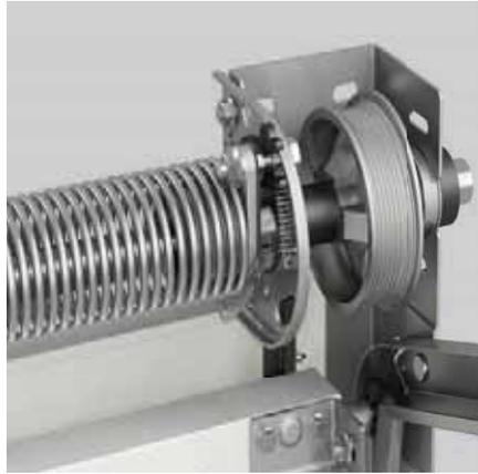
Torsion springs are equipped with **spring breaks** that stop the doors leaf from falling in the case of spring breakage. This protection system is supplied at no extra cost and ensures safe operation.
