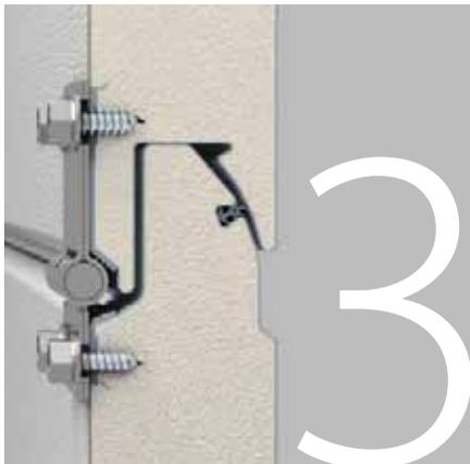
ALUTECH/GUNTHER sandwich panels have a closed loop design where steel sheets are interfixed into a «**lock**». This type of design prevents panels delaminating in the sun, or if the door meets a sudden obstruction. It therefore maximises the life span of the door, maintaining its smooth operation.
