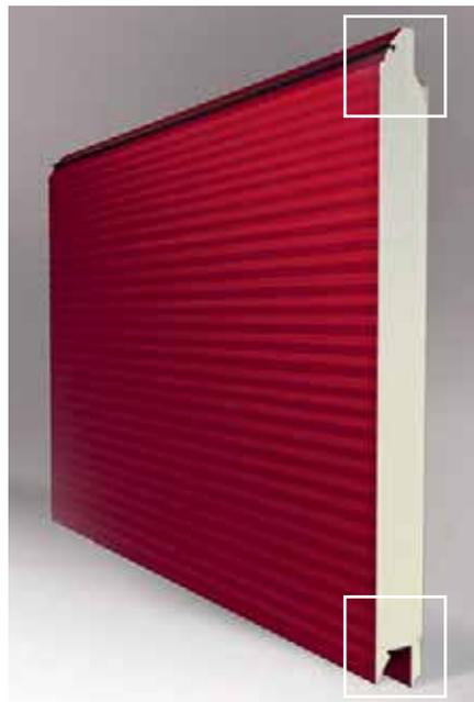
External and internal steel sheets of the sandwich panel are connected at the top and the bottom. Such a construction prevents panels from delamination caused by the heat of the sun, which is especially important for sunny locations and for dark coloured doors.
